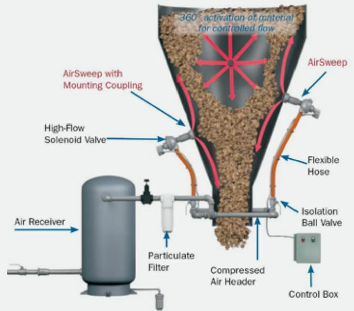
For the initial trial, two bins (9 feet wide, with 200-ton capacity) were hooked up to the [AirSweep VA-12 model 1 1/2" size Four AirSweep](#) were installed on each bin cone:
